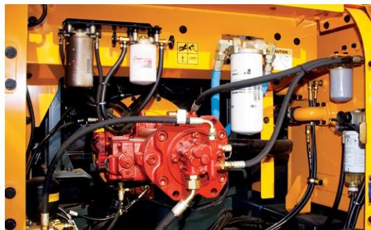
To achieve optimum precision, Hyundai redesigned the hydraulic system to provide the operator with super fine touch and improved controllability. Improved pump flow control reduces flow when controls are not being used to minimize fuel consumption.
