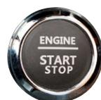
9A series excavators provide smart key system as an option. This allows the operator to start the engine by the push of a starter button without inserting a key in the ignition.
