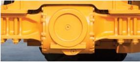
An enhanced axle improves driving over variable ground conditions. Self-adjusting brakes automatically regulate disc clearance, reduce service time and improve brake reliability and performance. The new load sensing hydraulic system with a variable displacement piston pump and closed center main control valve provide efficient hydraulic power and additional energy savings.
